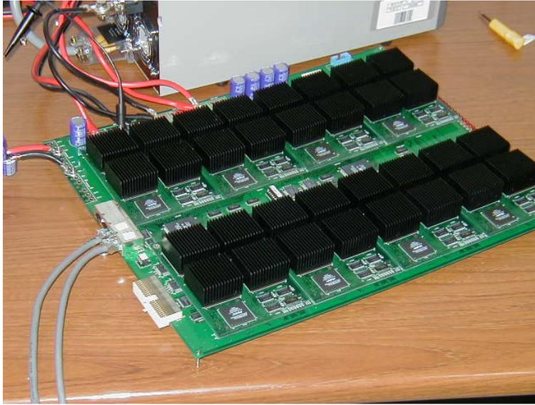
Figure 8: The GRAPE-6 processor board under testing.
