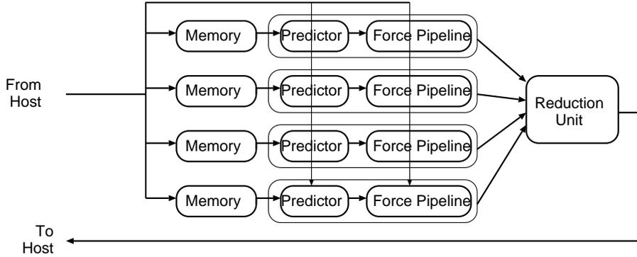
Figure 2: Parallel GRAPE pipelines for individual timestep algorithm.
