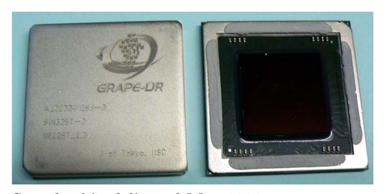
Sample chip delivered May 2006 90nm TSMC, Worst case 65W@500MHz
