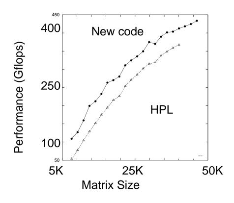
Speed in Gflops as function of Matrix size Top: new code Bottom: HPL 1.04a 430 Gflops (54% of theoretical peak) for
