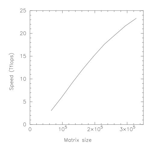
Measurement on 64-node, 48-Tflops system Matrix size limited by main memory size of host (18GB) Efficiency limited by matrix size...
