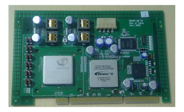
1st prototype board. (Designed by Toshi Fukushige) Confirmed succesful operation at 500MHz clock Currently working on softwares and FPGA design to run real applications
