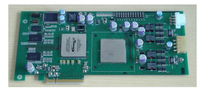
2nd prototype. (Designed by Toshi Fukushige) Single-chip board
