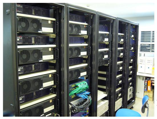
GRAPE-5 16 nodes (640Gflops peak) GRAPE-6 8 nodes (8Tflops peak) GRAPE-7 16 nodes (10Tflops peak)
